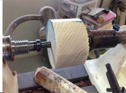
Remove the blank from between centers and Remount it into a scroll chuck --
