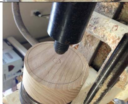
Before hollowing out the inside of the salt safe, I drill a hole, using a 1" forstner bit. Put a piece of tape on the forstner bit to mark the depth of the bottom. Working from the center out hollow out the interior of the box. I use a bedan for this, but a small 1/2 scraper will work just as well.
