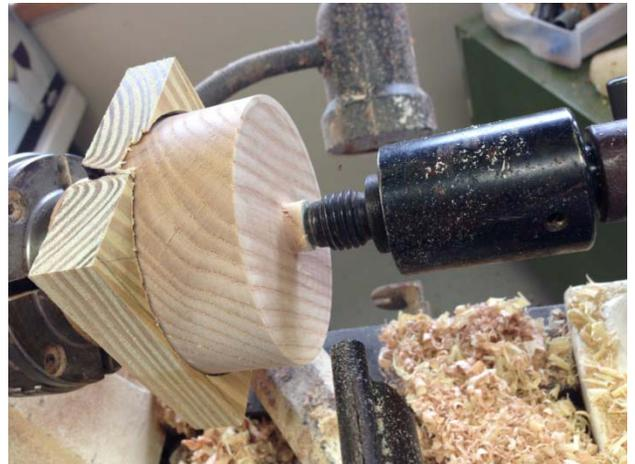
Drill holes for the magnets. I use 1/8 thick x 5/16" diameter magnets that I get from Harbor Freight. However, you can also find them on the internet. I use thin super glue to cement the magnets in place.
