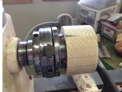
Mark off the top about 1/4 from the face and using a 1/16 or 1/8 parting tool part off the top.
