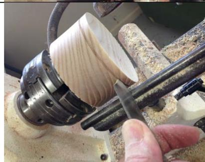
After the top has been parted off, remove the bottom from the chuck and again put it between centers, BUT, this time put it about 1/8 to 3/16" off center, and re-turn the tenon.
