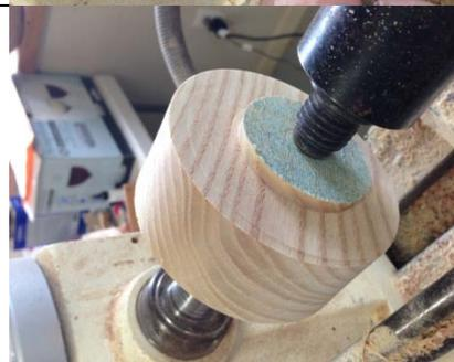
Remount the bottom in the scroll chuck and it will be off center. Make a pencil line around the top to see where the edges will be. Leave enough room for the magnet on the wider edge.
