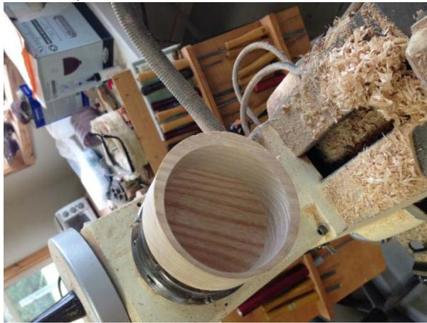
Remove from the scroll chuck. Make a jam chuck out of a scrap of wood turn off the tenon and finish the bottom.
